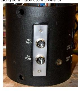
When mounted, the plate will have a gap around the sides and you will use clear silicone caulking to fill the gap. It looks rather hansom when finished.
