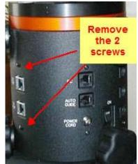
Now remove the 2 screws that hold the RJ45 connector boards.
