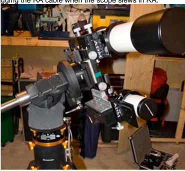
This is an extreme example, but this customer elected to use an alternate mounting location for his RA chassis connector to avoid the counter weight snagging the RA cable that would normally exit the side of the RA motor housing. In most cases, a right-angle plug would be sufficient.
