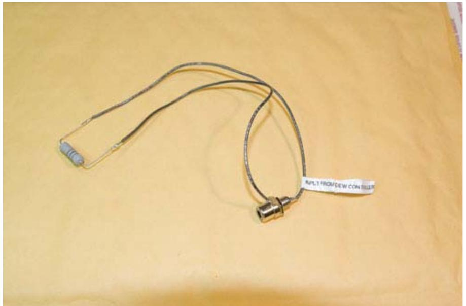
Do NOT connect directly to the heater. Like any other dew heater, you MUST use a controller. Do NOT connect directly to 12V or you will have a meltdown.
