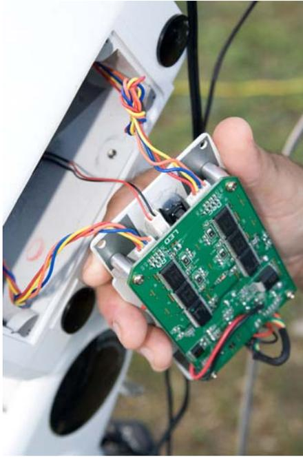
You will find 3 cables attached (RA & DEC motors and LED light for Polar Scope) to the circuit board attached to the inside of the panel plate. Label these cables and then unplug them.
