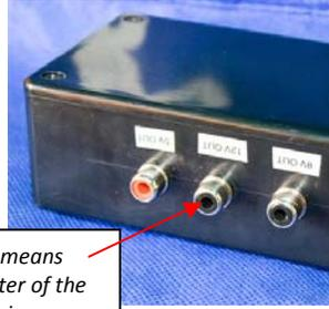
*Tip Positive* means that the center of the female chassis connector is + Positive
